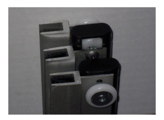
The following shows a right side view of the triple slide mechanism of the BBC Door, with the tracks slightly moved apart, corresponding with a mirror image of the triple slide mechanism shown in Figure 1 of the Patent:
