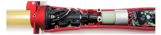
31. The following image of a dismantled Accused Product shows the terminal discs located between the bearing and the cylinder.
