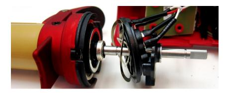
30. The following image of a dismantled Accused Product shows that it has a motor connected to the rotatable rod to rotate the cylinder:
