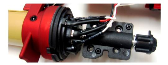
25. The following images of a dismantled Accused Product shows that it has a first terminal disc fixed to the cylinder and includes concentric annular electrical contacts:
