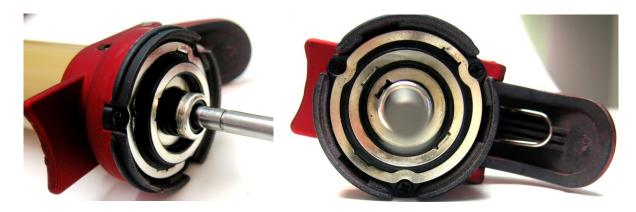
26. The following image of a dismantled Accused Product shows that it has a second terminal disc that is fixed relative to the body and includes concentric continuous annular electrical contacts:
