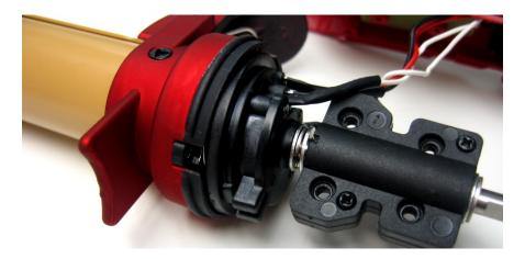
32. The following image of a dismantled Accused Product shows a thrust bearing affixed to the rotatable rod to prevent axial movement of the rotatable rod.
