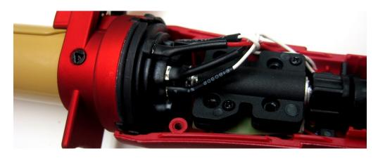
27. The following image of a dismantled Accused Product shows that the contacts on one of the terminal discs are bent upwardly and contacts on the other terminal disc are flat annular rings:
