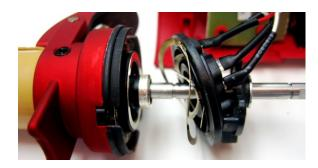
28. The following image of a dismantled Accused Product shows that the first terminal disc is held adjacent to the second terminal disc so that the contacts of the first terminal disc remain in contact with the contacts of the second terminal disc to provide an electrical circuit across the contacts to the heating element in the cylinder:
