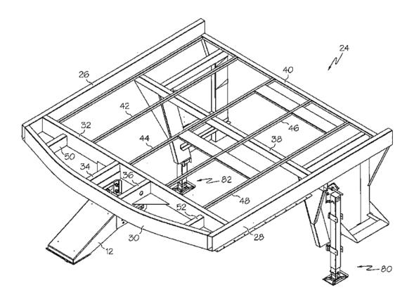
By comparison with prior types of chassis, the front end is formed with a curved or bent beam (denoted by number 30) connecting the side beams (denoted by the numbers 26 and 28).
