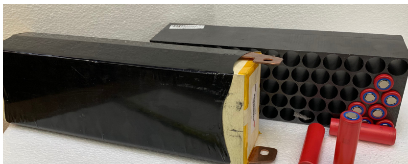
All Cell Thermal Management Blocks with Panasonic 18650 Cells
