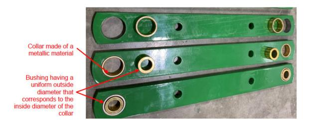
(Image of Arms from Solid Rock's Website www.solidrockag.com/parallel-arm-rebuilding)
